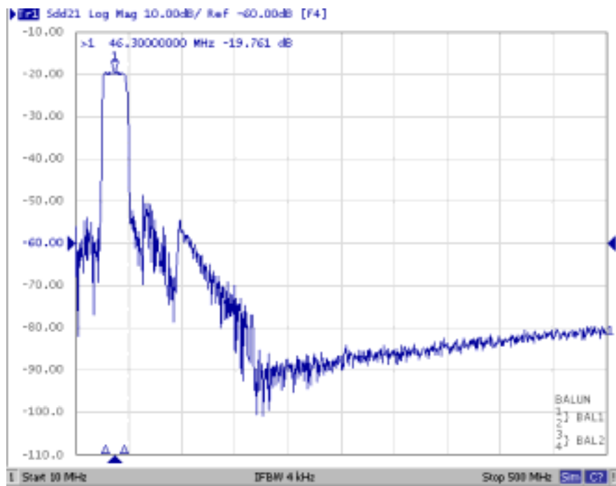
Fig1. Horizontal: 50MHz/Div Vertical: 10dB/Div
