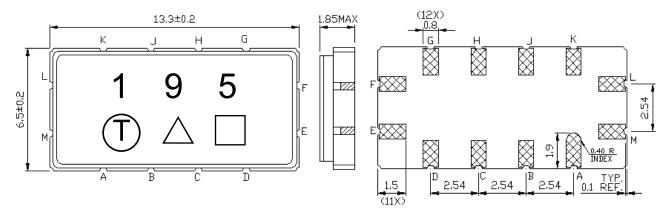
Pin L: RF Input Pin E: RF Output Pin M: Input Ground Pin F: Output Ground Pin A, B, C, D, G, H, J, K: To be Ground Unit: mm  $\triangle$  : Product / Year Code  $\square$  : Week Code
