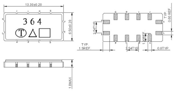
Pin K=L: RF input Pin E=F: RF output
