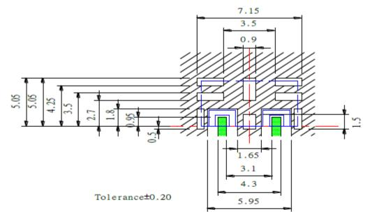
Conductive Material: Ground, connected to lower ground diameter of 0.3mm and max.distance of 1.0mm.
