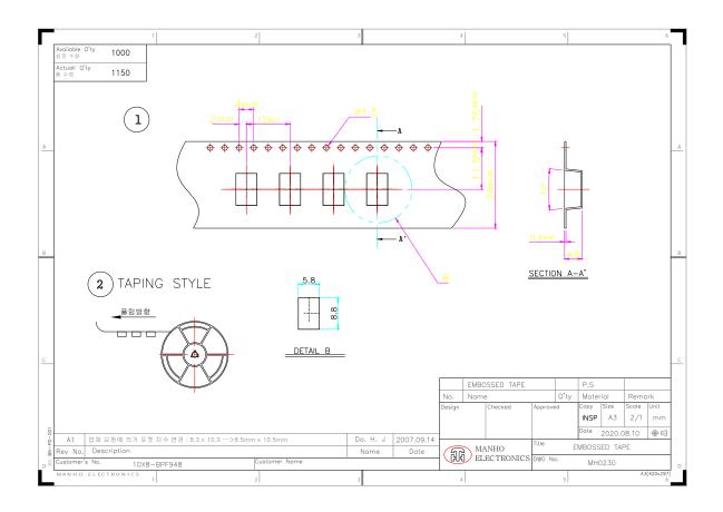
Figure 4. dimensions of carrier tape
