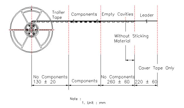
FIGURE 6. Taping Conditions.
